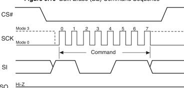
Figure 9.10 Bulk Erase (BE) Command Sequence
