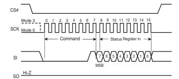
Figure 9.7 Write Status Register (WRSR) Command Sequence
