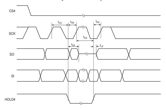
Figure 16.4 Write Protect Setup and Hold Timing during WRSR when SRWD=1
