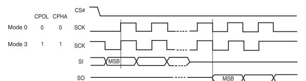
Figure 6.2 SPI Modes Supported
