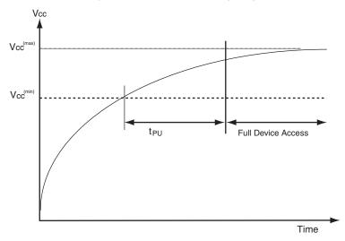
Figure 10.1 Power-Up Timing Diagram
